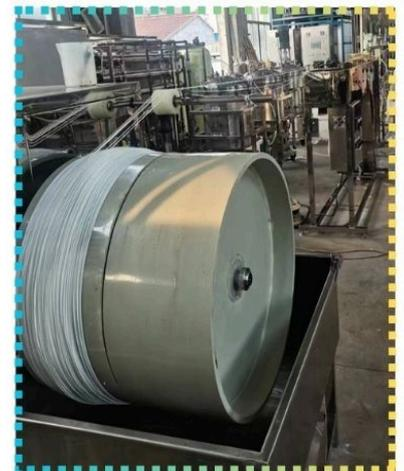
Large Scale Spinning line - Hollow Fiber Membranes
